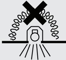
Ensure free movement of air around the fitting by removing any roof void insulation from at least 150mm around the hole. Under no circumstances must these fittings be covered with insulating matting or similar material.
