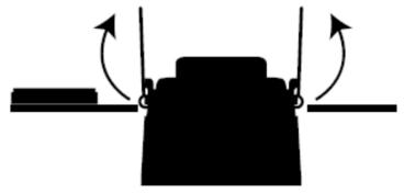
Fold spring clips upwards and insert fitting into hole
