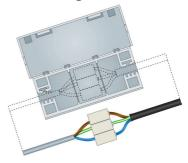
7. Push the cables down into the clamps as far as they will go. Close the lid and snap shut.
