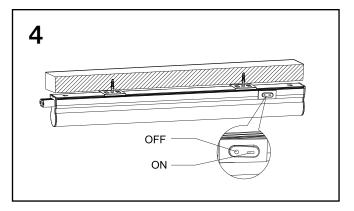
3). When the fixings are secure, locate the base of the luminaire into the mounting clips.
