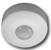
This product uses an infra-red heat detector. The detector senses 'warmth movement' in the surrounding area when it is dark. When movement is detected the sensor is activated and triggers the connected load. It has a built in photo-cell that can identify day and night.
