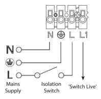
**Note:** Any floodlight connected to the L1 Switch Live terminal 'Live Output' will be controlled by the PIR
