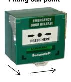
Lift front of unit up from bottom and slide to one side to open the unit
