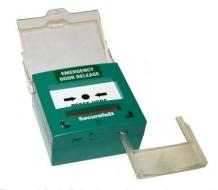
For semi-flush fitting insert key as shown and twist clockwise in slot to remove call point from back plate.
