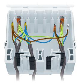
6. When a large number of cables need to be connected on a single circuit then the central receptacle can be used to connect the cable earth wires together using the 2273-208 PUSH-WIRE® connectors and jumper bar 862-482.
