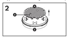
Loosen but do not remove the gear tray retaining screws 3. Adjust the position of the gear tray to align the hole in the keyhole slots with the retaining screws. Remove the gear tray 4 from the base 2.
