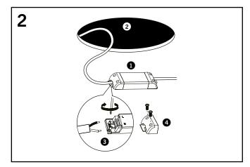
Locate the LED driver ① which is supplied with the luminaire into the open ceiling void ②. Connect the mains supply cable to the LIVE and NEUTRAL input terminals ③ and replace the terminal cover cap ④. Ensure that the correct polarity is observed.
