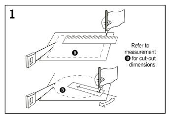
Decide the mounting position and accurately cut out the mounting hole in the ceiling. Do not exceed the relevant cut out dimensions and ensure that each luminaire is spaced adequately to provide clearance from any joists, beams or cables within the ceiling void.
