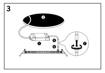
Connect the plug lead **5** which is pre-wired into the output terminals of the LED driver **1** to the lead which is attached to the luminaire **6**. Rotate the two plugs 90 degrees to ensure a secure connection **7**.
