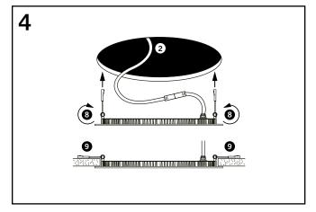
With the spring clips held in the upward position ③, insert the luminaire through the cut out hole and into the ceiling void ②. Take care not to trap any loose cables. The spring clips will locate onto the top of the ceiling surface to provide a secure installation ④. Ensure that the luminaire is fitted centrally to the cut out mounting hole.
