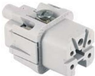
Female insert, JK series, screw terminal connection, 4 poles + PE, 10 A 230/400 V 4 kV 3, size "21.21"
