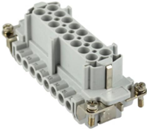
Female insert, JNE series, screw terminal connection, 16 poles + PE, 16 A 500 V 6 kV 3, size "77.27", with plate
