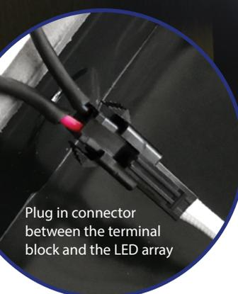
Plug in connector between the terminal block and the LED array
