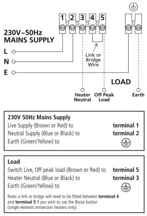
230V 50Hz mains – Twin or Dual element immersion heaters.
