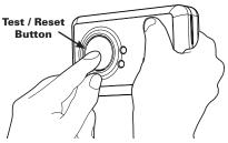
Cover the sounder vents with one hand. Press and hold the Test/Reset button down with your thumb/finger until the Power LED illuminates green and the sounder sounds for a second time (this should happen after around 5 seconds). Release the Test/Reset button. Upon releasing the Test/Reset button the Power LED will flash green once every second. This indicates that the sampling rate of the detector has increased and can be tested using a known source of CO.
