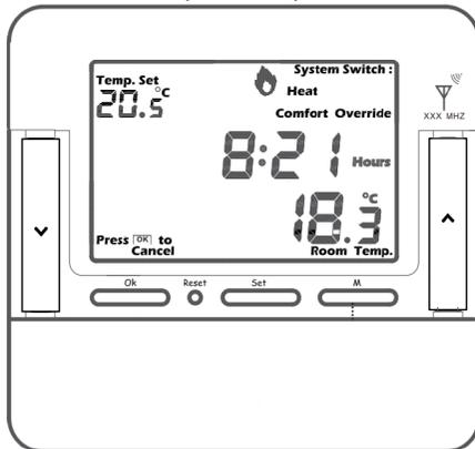
**Comfort Override** is shown above the time on the display. Time changes to countdown of the remaining hours and minutes.
