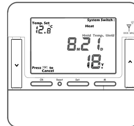
**Hold Temp. Until** is shown above the date on the display. Bottom right cycles between the set year and the room temperature.
