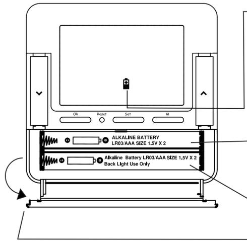
When the Battery Low warning sign appears on the display, replace the batteries immediately.
