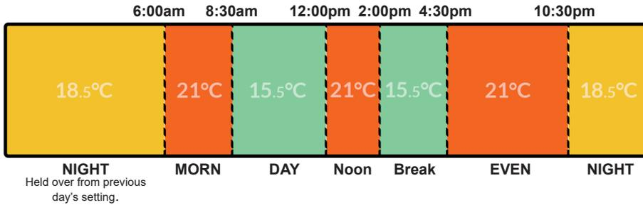
Essentially, if the thermostat reads the temperature below the chosen temperature it will send a message for the boiler to fire and your heating to come on.
