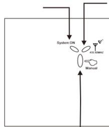
If LED is permanently lit no RF signal is being found. Heating will turn off after 10 minutes if no RF transmission resumes. After the RF signal is recognised the heating schedule will continue.
