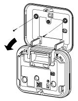
Flip down the CO alarm, away from the bracket. Please ensure that you use the screws provided, as they were chosen specifically for use with this product. Drill holes into the wall. Insert the plastic wall plugs. Using a screwdriver push out the plastic knockouts in the bracket (see illustration). Using the holes as a guide, drill the screws through to secure the bracket in place.
