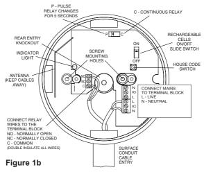
If momentary relay operation is required, carefully and gently slide the yellow switch to the "P" position with a small screwdriver (see figure 1b). This is commonly used with warden call systems where only momentary short circuit signalling is required. This must be done before the mains power is connected or the rechargeable cells are activated. With the switch in the "C" position, the alarm signal will switch the latching relay until it receives a cancel signal.
