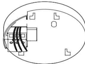
If the mains wires are being brought along the surface, break the knockout and trim to accommodate the conduit.
