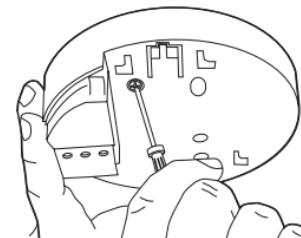
Slide Alarm on to the Ei168RC RadioLINK Base. This will automatically activate the rechargeable back-up cells in the base.
