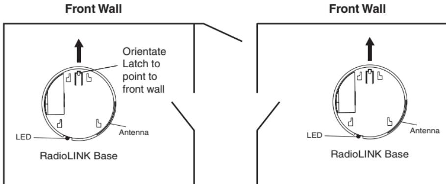
**Orientate all RadioLINK bases in the same direction**
