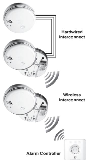
In this configuration the alarm controller must be a RadioLINK device.
