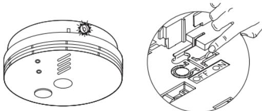
Press and hold the test button. The red led will flash and the horn will sound.
