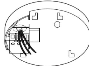
Screw the base to the ceiling using a single screw for now. The second screw should be inserted at the end of this procedure to secure the base permanently.
