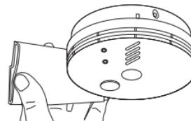
Vacuum all around the smoke entry openings in the smoke Alarms to remove any excess dust, lint, cobwebs, etc.
