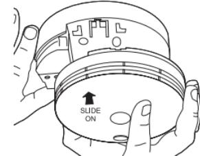
If the blue light flashes every 10 seconds, remove the alarm and manually depress the rechargeable cell "on" switch as shown and refit the alarm. If there is still a problem the cells may be depleted so leave the unit on mains power for 2 hours to charge and test again.
