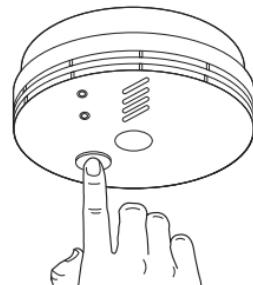
**DO NOT TEST WITH FLAME** (this can set fire to the Alarm and damage the house).
