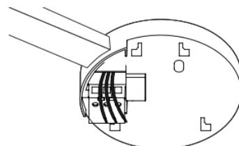
To prevent air draughts affecting smoke or heat entering the alarm it is important to seal the area around the hole in the ceiling with foam or silicon rubber.
