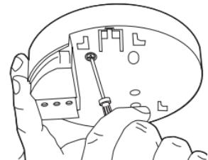
Connect the wiring to the terminal block as shown here.
