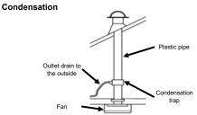
To avoid the backflow of condensation into the fan in ceiling installations it is good practice to fit a condensation trap to the vertical outlet duct of the fan. With thru-the-wall installation fit the duct in an approx. 5° angle down to outside.
