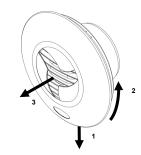
To remove front cover assembly, first make sure the fan is off. isolated from the power supply and the iris shutter is fully closed.
