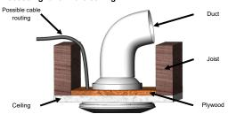
The fan should be fitted in the hole, fixed with the screws provided into the support.
