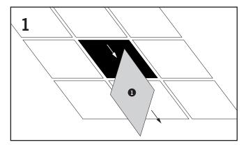
Always switch off / Isolate the mains power supply before installation or servicing. When installing into a suspended ceiling grid, remove the tile or tiles **1** from the position where the LED Panel is to be located.
