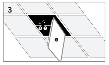
Connect the driver plug lead **4** which is pre-wired into the output terminals of the LED driver to the panel plug lead **5** which is attached to the LED Panel **6**. Rotate the two plugs 90 degrees to ensure a secure connection.
