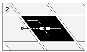
Locate the LED driver ② into the open ceiling void and connect the mains supply cable ③ to the input terminals of the driver. Ensure that the correct polarity is observed: LIVE (L) Brown to terminal marked L – NEUTRAL (N) Blue to terminal marked N
