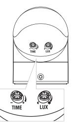
Note: when testing in daylight, please turn LUX knob to - + (SUN) position, otherwise the sensor lamp could not work!
