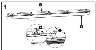
Isolate the mains power supply before commencing installation. To access the luminaire interior, lift and release the steel clips 1 on each side of the base 2 and remove the diffuser 3
