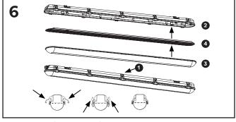
Refit the gear tray 4 onto the base 2 and ensure that it is securely fixed onto the spring fixing clips 5. Replace the diffuser 3 and ensure that all the steel clips 1 are securely fastened to maintain the IP65 rating.
