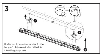
Mark and drill 2 fixing holes for the surface mount brackets provided **7**. Mount the brackets securely to the ceiling at the correct fixing centres (LF) for the version being installed (see table for LF). Offer the base **2** up to the brackets **7** and push to `Snap fit`
