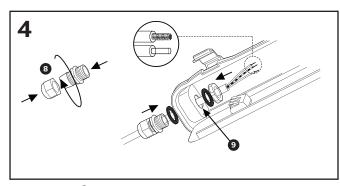
Fit the cable gland ⓐ and mains supply cable through the cable gland entry point at the end of the base ⑤. It is the installer`s responsibility to ensure that the gland is correctly fitted to maintain the IP65 rating
