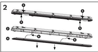
Remove the gear tray **4** from the base **2** by pressing the spring fixing clips **5** inwards. Retaining straps **6** prevent the gear tray from falling during installation and servicing
