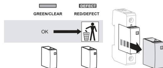
Where surge protective devices (SPDs) or other equipment are likely to influence the verification test, or be damaged, such equipment shall be disconnected before carrying out the insulation resistance test.
