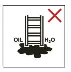
Do not erect ladder on contaminated ground
