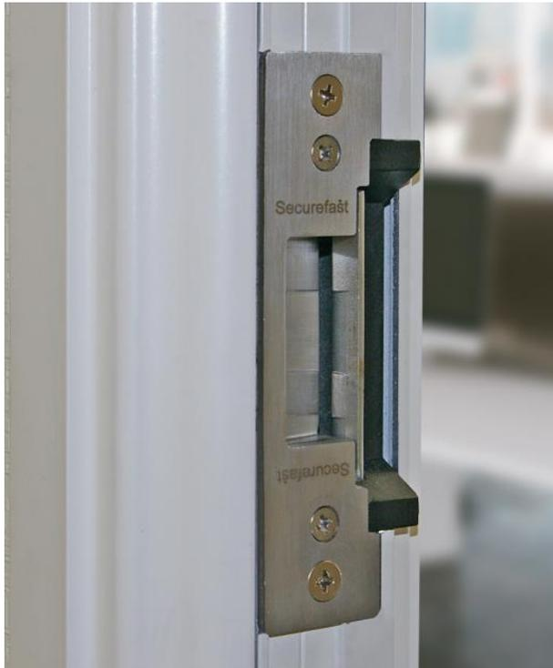
*The AL900 series electric releases are an ANSI style door release, complete with stainless steel short or long faceplates for use in metal or timber frame applications. The electric releases are designed to work with most leading brand mortice nightlatch locks.*
