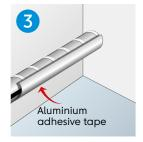
For plastic pipe and plastic components the trace heating cable must be wrapped with an aluminium adhesive tape.
