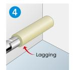
After installation of the trace heating cable, the pipes must be insulated with a minimum of 20mm lagging (Armaflex/PU Foam/Mineral Wool).
