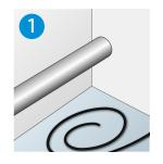
Roll out the trace heating cable. Avoid bending the heating cable beyond the minimum bend radius.
