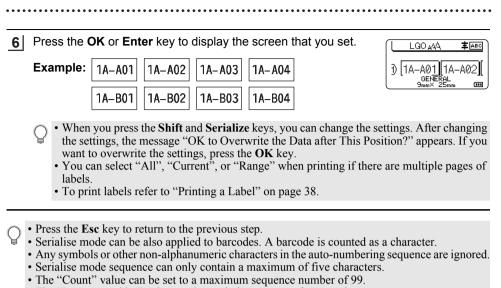
• The "Incremented by" value can be set in increments of one to nine.
