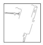
**Step 4.** Raise the heater to upright position. Present the heater and engage 2 slots of the bottom parts of the wall brackets in the wall heater's rear enclosure then pull up the heater. Then engage 2 slots of the upper parts of the wall bracket and tighten the 2 screws in order to lock the device.
