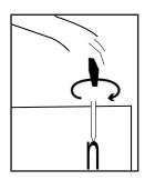
**Step 2.** Then pull out the top bar by pressing firmly both upper parts slotted into the rear housing. Slide down the wall bracket in order to remove it from the rear housing.
