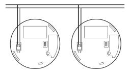
A maximum of 250 meters of two core,  $0.5mm^2$  to  $0.75m^2$ , stranded signal cable can be used (maximum resistance between detectors 50 ohm).
