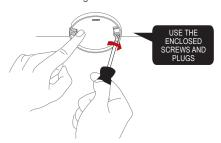
Once the mounting base is installed, attach the alarm by twisting clockwise until it clicks. If the switch is in 'Learn Mode', the smoke alarm will not be able to click into the mounting base.
