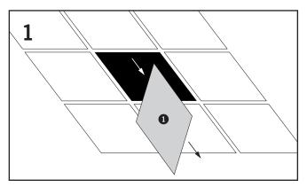
Always switch off / Isolate the mains power supply before installation or servicing. When installing into a suspended ceiling grid, remove the tile or tiles **1** from the position where the LED Panel is to be located.
