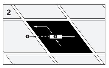
Locate the LED driver ② into the open ceiling void and connect the mains supply cable ③ to the input terminals of the driver. Ensure that the correct polarity is observed: LIVE (L) Brown to terminal marked L – NEUTRAL (N) Blue to terminal marked N
