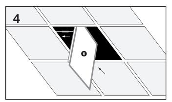
Place the LED Panel ③ into the open ceiling void and locate the panel frame onto the exposed T bar grid. Restore the mains power supply, switch on and test for satisfactory operation.
