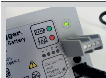
Fig 63: Battery pack connected
