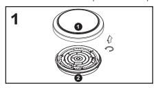
Remove the front diffuser/decorative trim ① from the base ② by rotating 45 degrees anti-clockwise and pulling away from the base tray.
