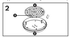
Loosen but do not remove the gear tray retaining screws ③. Adjust the position of the gear tray to align the hole in the keyhole slots with the retaining screws. Remove the gear tray ④ from the base ②.
