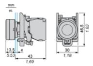
e : clamping thickness: 1 to 6 mm / 0.04 to 0.24 in.
