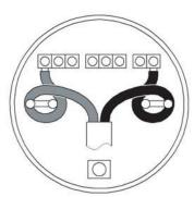
After wiring the ceiling rose & before fitting the cover, ensure both the wires to the pendant fitting are routed around the cable restraint posts as shown in diagram. This must be done to avoid the weight of the pendant & any lamp shade putting undue strain on the terminal connections.
