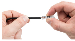
Insert the conductor.
