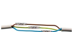
Strip 10 mm conductor per specification and insert connector (example shows staggered connectors).
