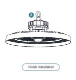
$\label{eq:WARNING: The sensor must be correctly tightened to make it waterproof.}$
