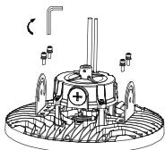
Align the 2x smaller brackets together with the main surface bracket. Fasten tightly using the 2x M5 screws and 2x M8 screws.
