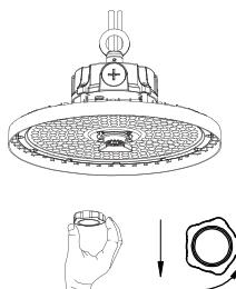
Install sensor into the socket.
