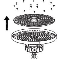
**Important** - Remove the 2x seal rings from the old lens. Insert them carefully into the same positions on the new lens
