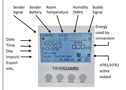
To power the PV monitor, connect the USB cable supplied with the unit to a suitable 5V USB power supply.
