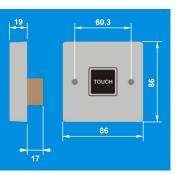
**ELLIPSE** Push button activated time lag switch **KH2** Touch activated time lag switch The ELLIPSE and KH2 time lag switches are a quick and effective way to reduce energy consumption for lighting applications. Pressing the button or touch pad brings the lights on; the lights will then switch off automatically after a preset time period has elapsed.
