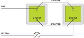
WIRING DIAGRAM FOR TWO WAY SWITCHING USING TIME LAG SWITCHES
