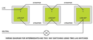
WIRING DIAGRAM FOR TWO WAY SWITCHING STRAPPER
