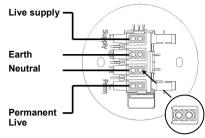
Each pole has **two** screw terminals. Each terminal accepts 1 x 2.5mm<sup>2</sup>
