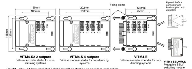
Height - allow 150mm for total height of unit (including connectors and cable)
