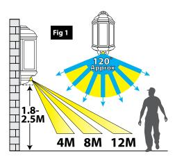
To avoid damage to the unit do not aim sensor towards the sun.
