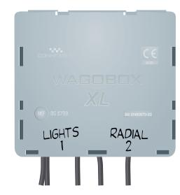
5. When two separate circuits are being supported no connections between the left and right side are permitted. Each side must be dedicated to one circuit
