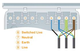
2. Prepare the cables by **stripping back 70 - 80mm of the outer sheath.**
