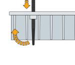
13. If required the WAGOBOX can be fixed to a surface using the fixing button feature. Simply fix the button in the required position and slide the WAGOBOX into place using one or both of the fixing slots in the base.
