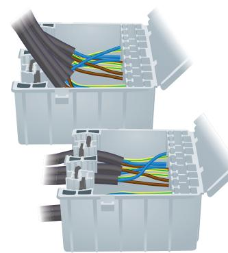
10. Then simply slide the cables down into the gripper slots.
