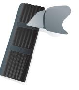
8. Install the largest cable at the bottom of the gripper slot first. Then the next size on top and the smallest last. Fit the gripper first, then each section of cable in turn to prevent the cables moving up the gripper slot.
