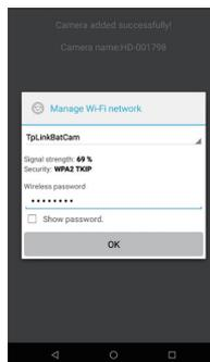
Then your Wi-Fi list will popup out, please select your home network from the menu and then enter your home network's wireless password Tap OK. The camera will be off-line for around 90 seconds to reboot for the connection to establish. When the camera connects to Wi-Fi router successfully, the Blue LED will be constant.
