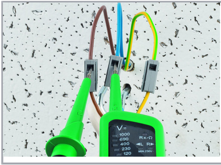
Testing via separate test ports.
