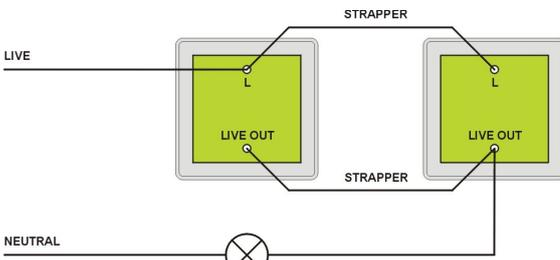
WIRING DIAGRAM FOR TWO WAY SWITCHING USING TIME LAG SWITCHES
