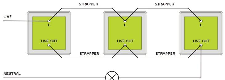
WIRING DIAGRAM FOR INTERMEDIATE AND TWO WAY SWITCHING USING TIME LAG SWITCHES
