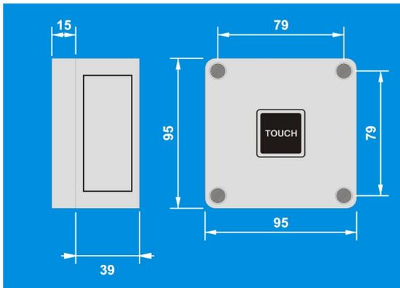
The KH3 time lag switch is a quick and effective way to reduce energy consumption for lighting applications. Pressing the touch pad brings the lights on; the lights will then switch off automatically after a preset time period has elapsed.
