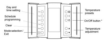
\* Use this button to disable heating (e.g. in the summer). The thermostat remains powered and continues to display the time and temperature.
