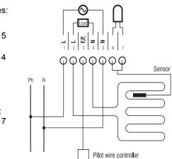
**WARNING:** Ensure that the wires are tightly secured to the terminals. Apply a minimum torque of 0.5 Nm (4.4 Lb/in) when tightening the screws.
