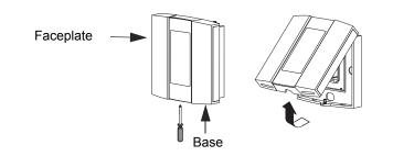
Before making the connections, make sure that the base covers the electrical box entirely. If not, install a wall plate at the back of the base.
