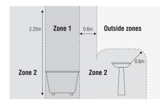
This product is suitable for use in Zone 2 and outside Zones of a bathroom. See diagram. If this unit is being fitted in a room containing a bath or shower, a 30mA RCD must be used, in accordance with IEE regulations.
