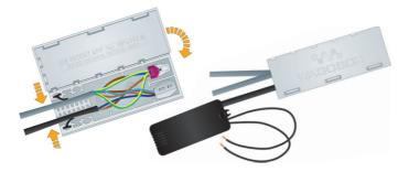
8. If required the WAGOBOX® can be fitted to a surface using the mounting button. (sold separately, part No. 51009130 pack of 10)
