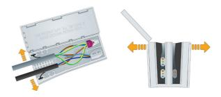
7. Try to keep cables of a similar size together in the same slot and simply push them into the slot as far as they will go.
